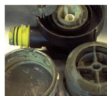
Centrifuge housing, encrusted - total breakdown of the suction machine
