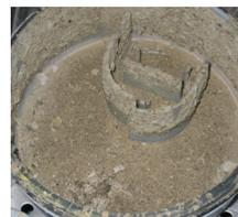
Separation tank, full of sludge
